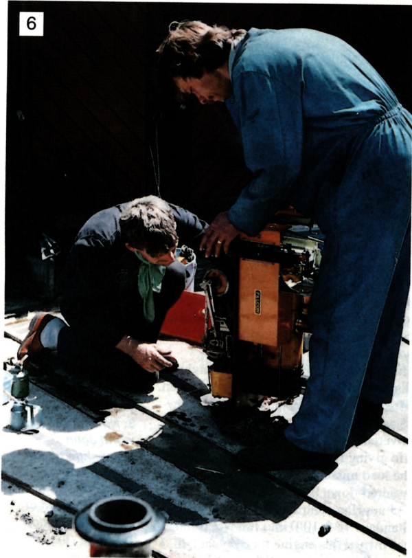
6: One beauty of the little 'uns is that they can be up-ended for routine chores such as oiling up. Stuart Duncan holds Tich, whilst John Painter checks the between the frames workings, prior to his run.
